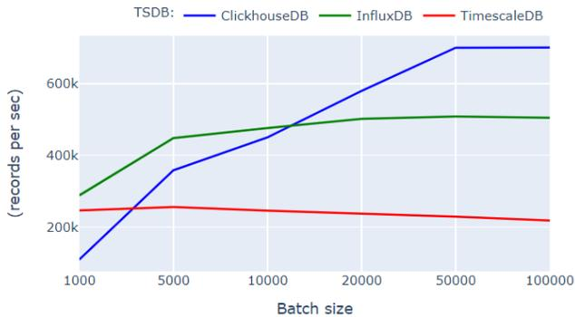
Figure 29 - Ingestion rate mean per batch size with 12 clients
