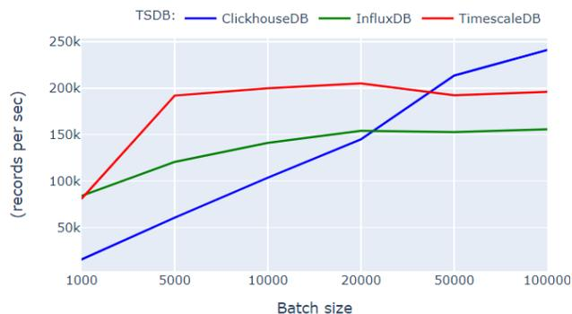
Figure 27 - Ingestion rate mean per batch size with single client
